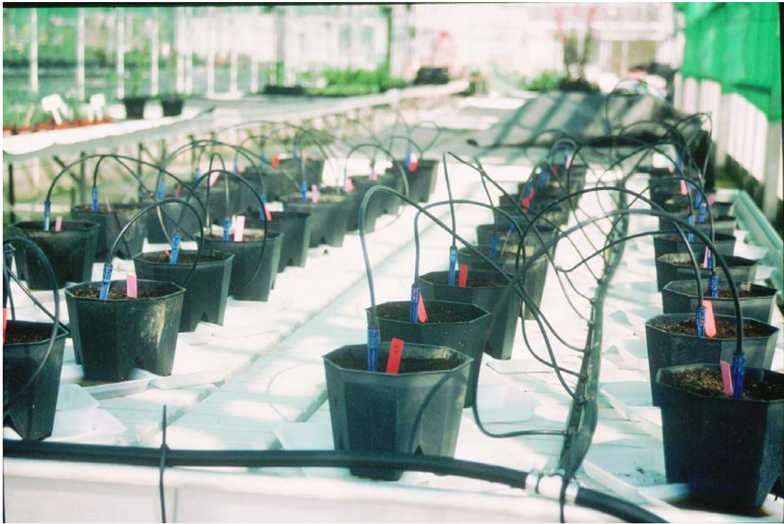
Photos 5 and 6 Testing horizontal distribution of water from a dripper
